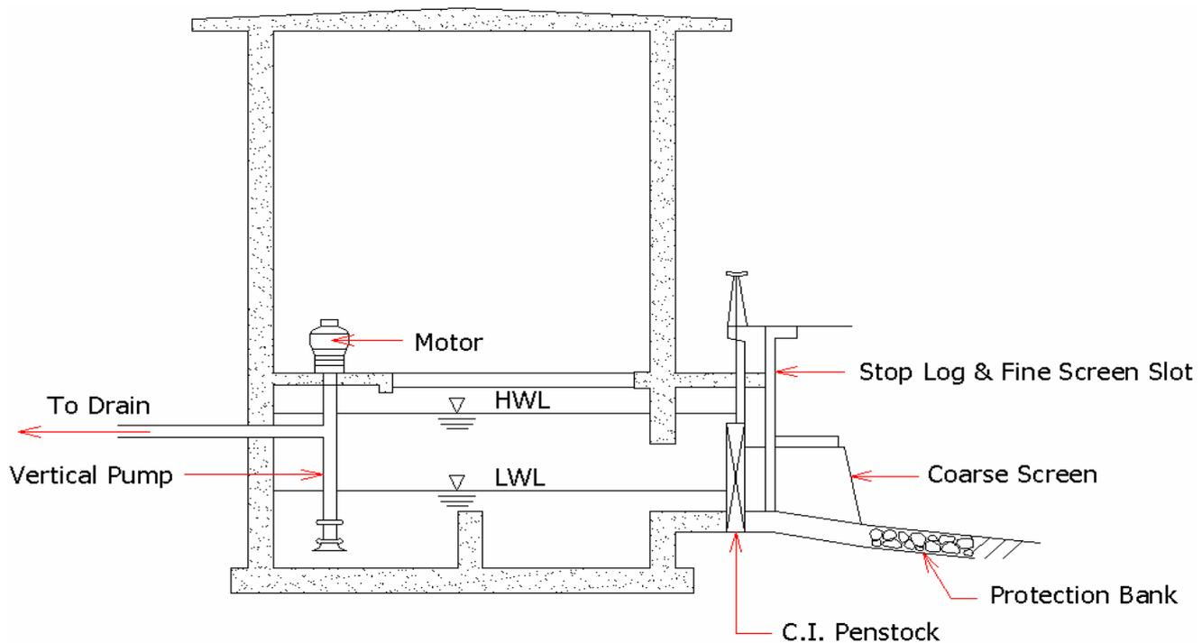
Figure 45.1 Typical Wet-pit Station
