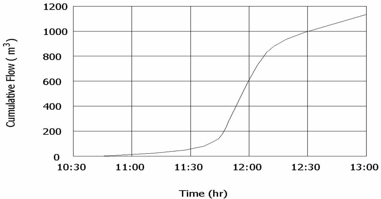
Figure 45.6 Estimated Required Storage from Inflow Hydrograph.
