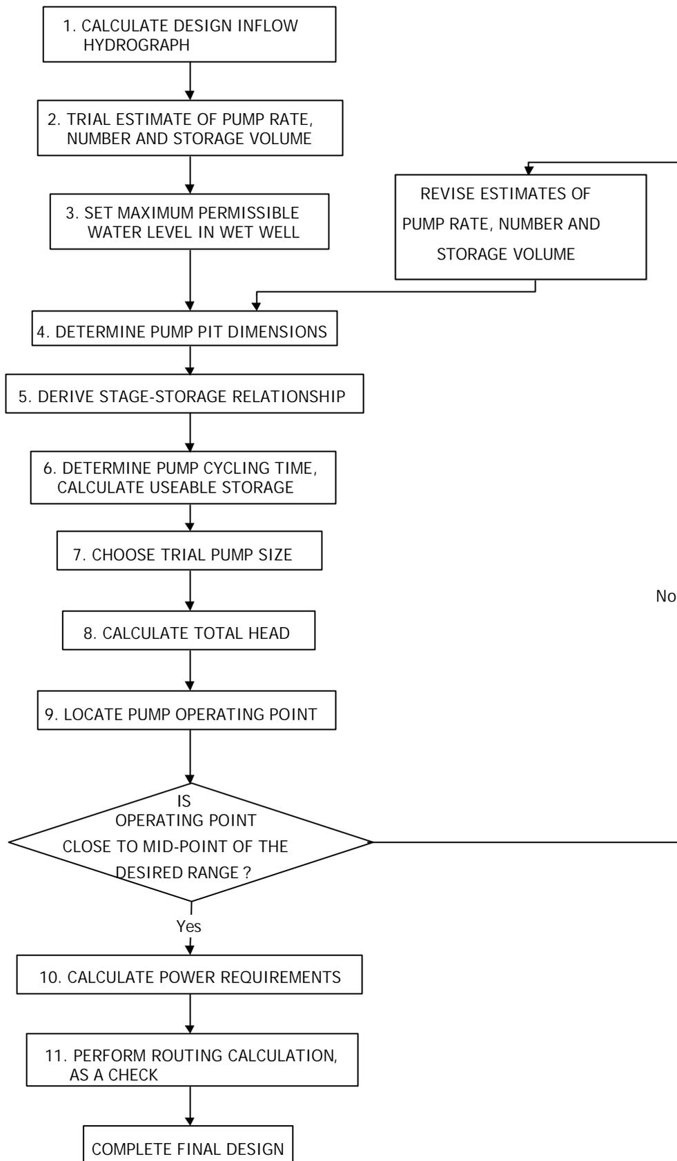
Figure 45.8 Flowchart for Pump Station Design
