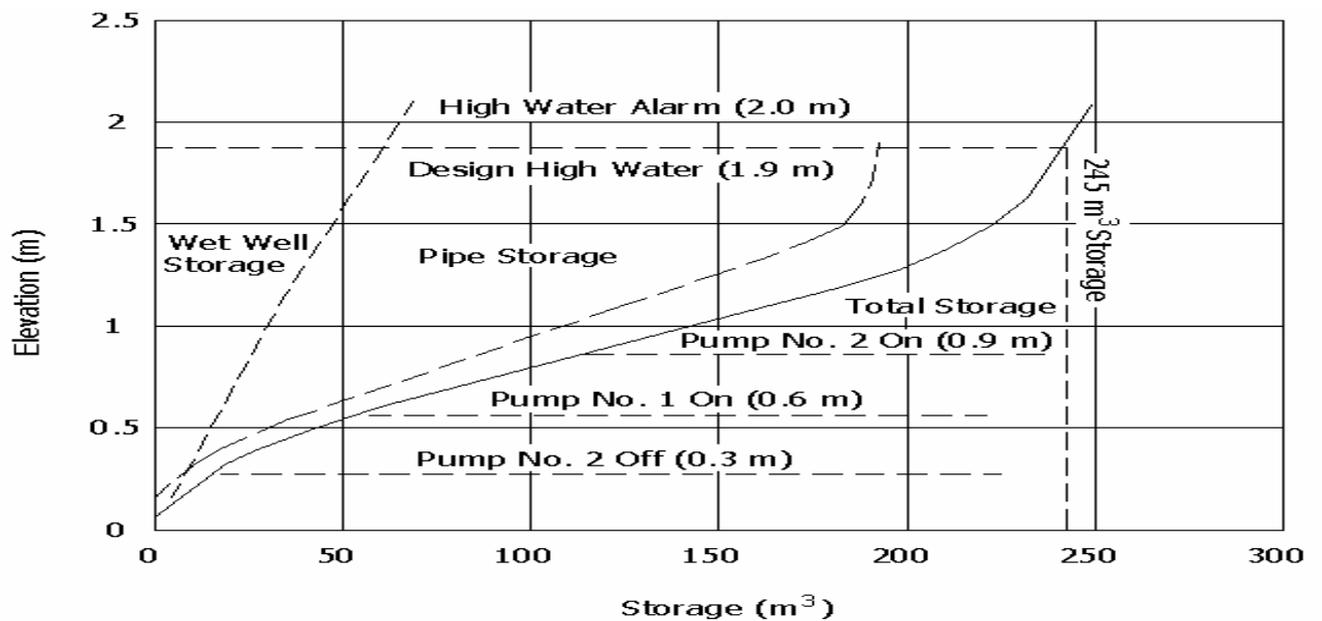
Figure 45.A6 Stage-storage Curve for Example 45.A.2.
