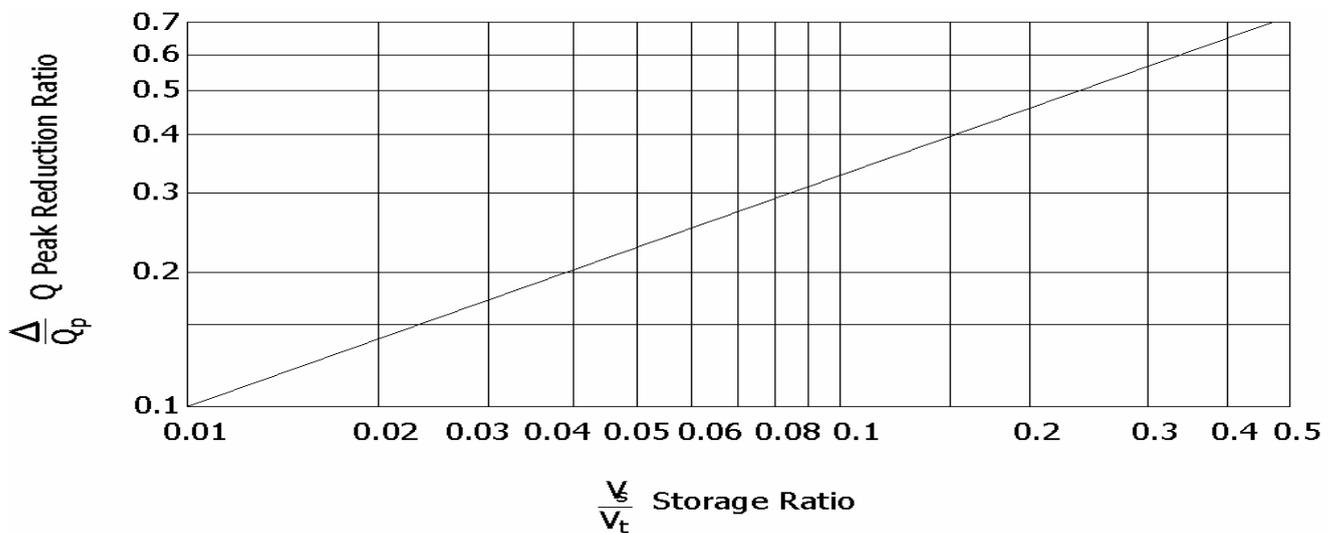
Figure 45.A3 Relationship between Peak Reduction Ratio and Storage Ratio :  $V_s/V_t = (\Delta Q/Q_p)^2$  (Baumgardner, 1981)
