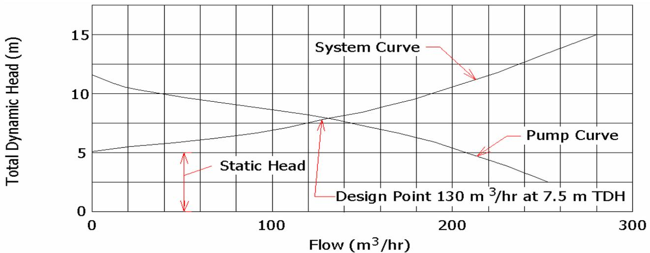
Figure 45.4 System Head Curve
