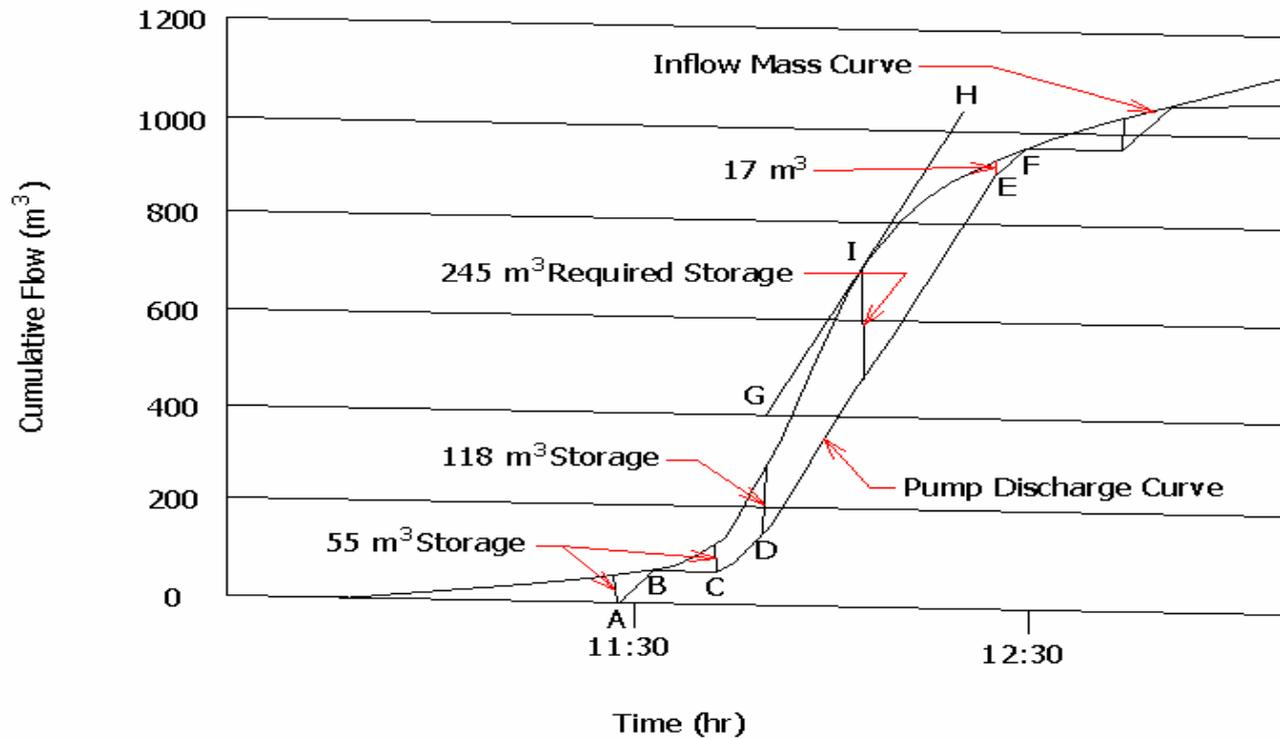
Figure 45.A8 Mass Curve Routing Diagram
