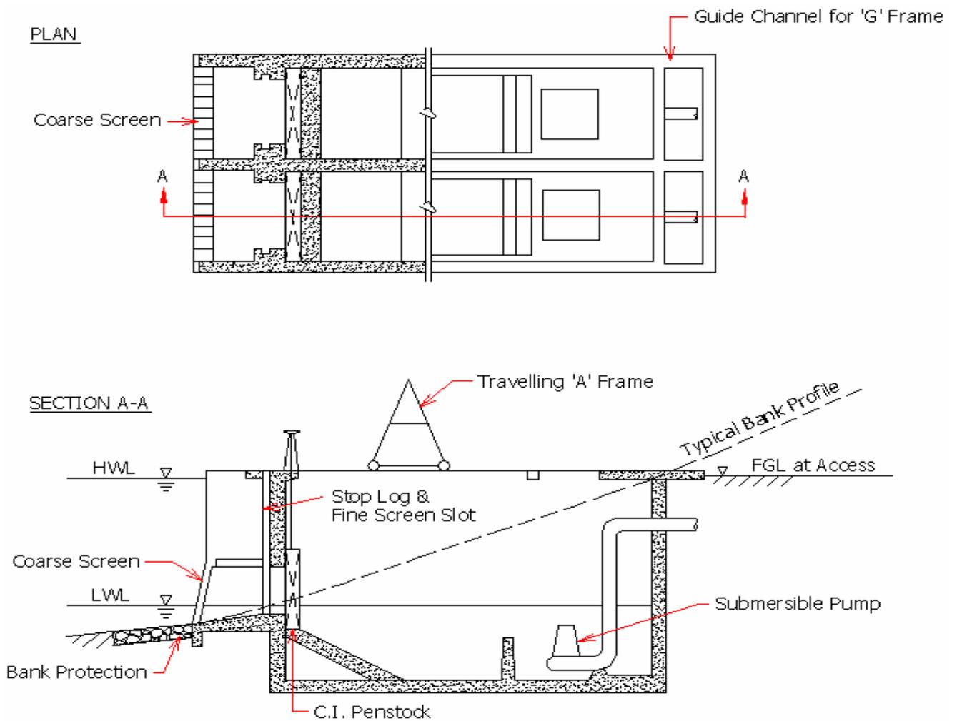
Figure 45.3 Typical Submersible Stormwater Pump
