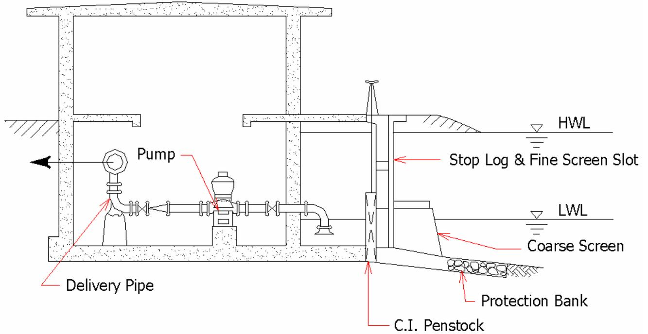
Figure 45.2 Typical Dry-pit Station
