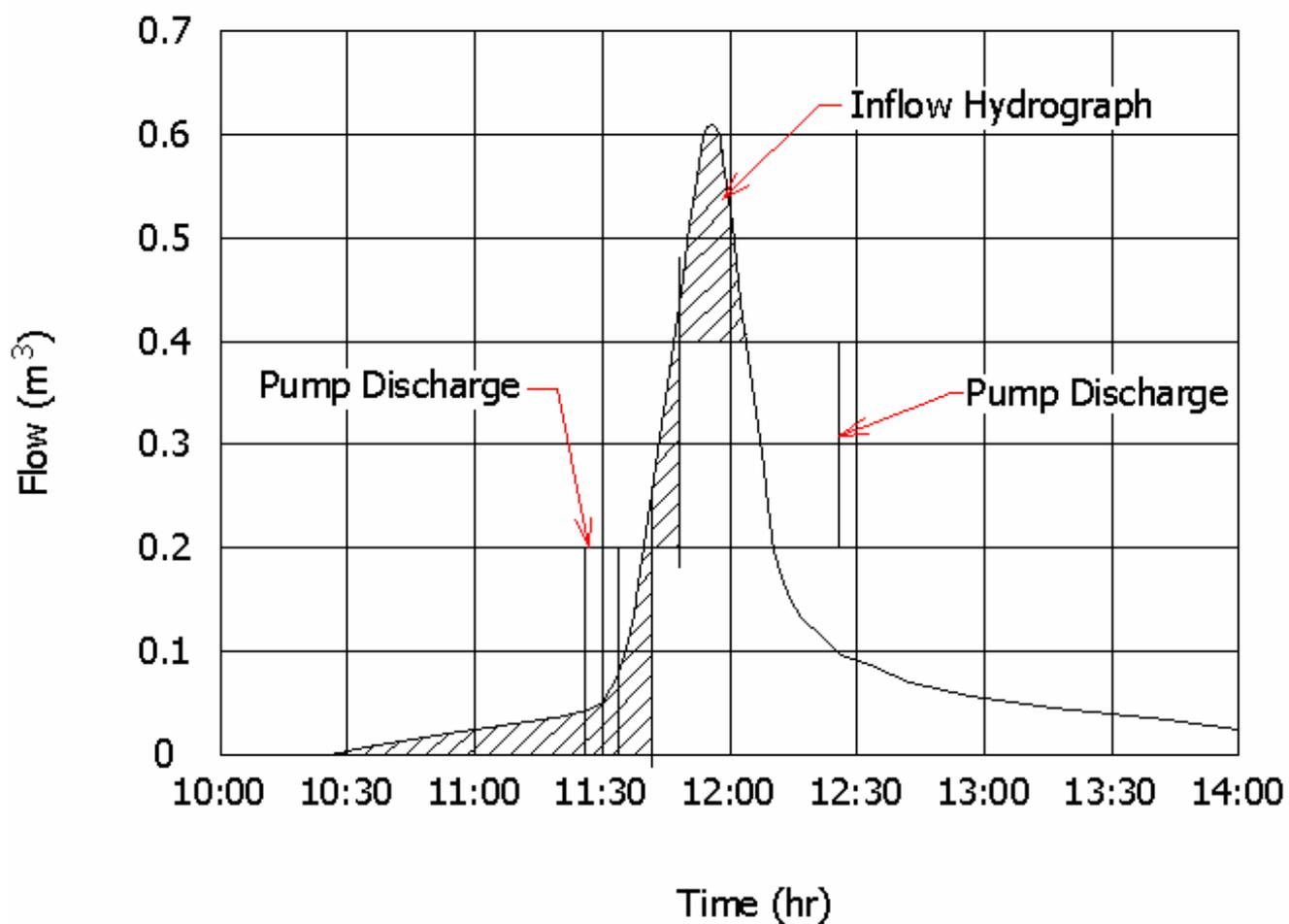
Figure 45.A9 Pump Discharge
