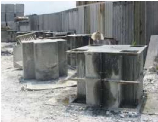
I. Casting of VIP LINER at Factory
