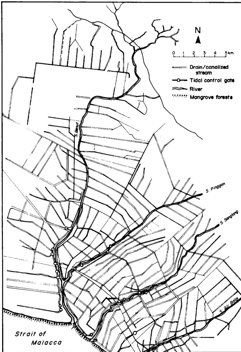
Fig. 2. Drainage controls in Sg. Benut catchment.
